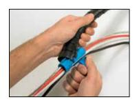
Place the applicator tool in one end of the Helawrap sleeving.
