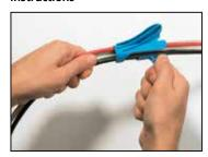
Insert one or more cables into the insertion slot of the applicator tool.
